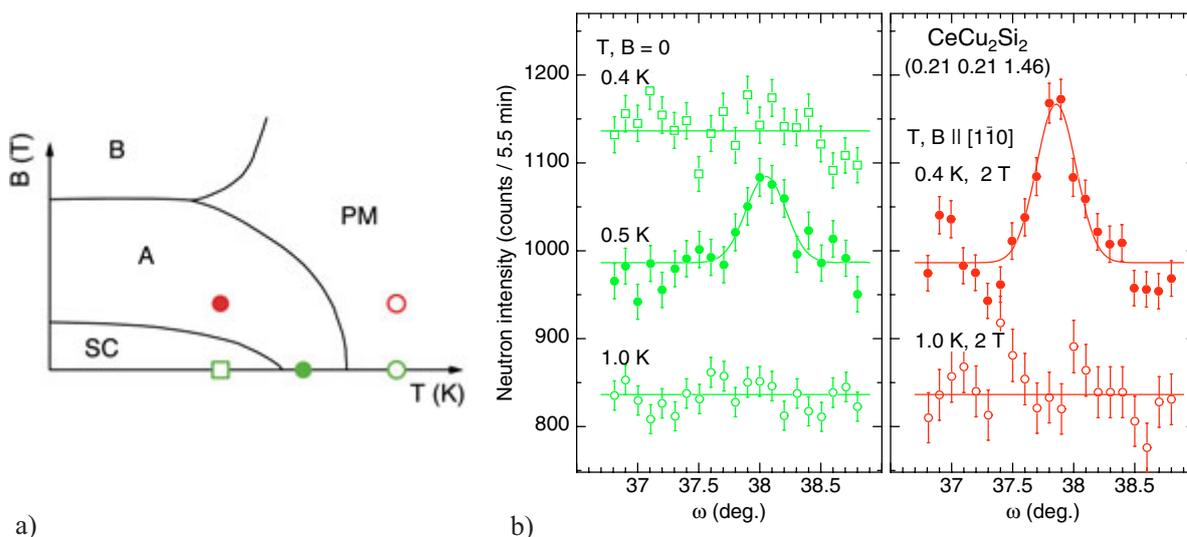
Fig. 2: (a) Schematic magnetic  $(B, T)$  phase diagram of  $\text{CeCu}_2\text{Si}_2$  with different magnetically ordered phases (A-, B-phase) and the superconducting phase. The  $(B, T)$  values at which neutron diffraction measurements were performed, are marked. (b) Rocking scans across the position of a magnetic superstructure peak in an A/S- $\text{CeCu}_2\text{Si}_2$  single crystal at different temperatures and magnetic fields [8].
