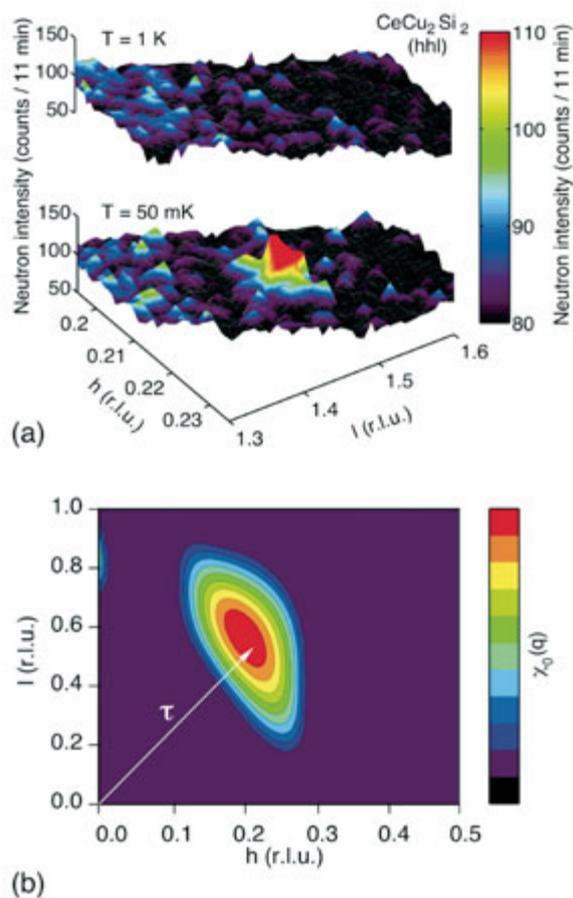
Fig. 1: (a) Intensity map of the reciprocal (*hhl*) plane around  $q = (0.21 \ 0.21 \ 1.45)$  in  $\text{CeCu}_2\text{Si}_2$  at  $T = 50$  mK and 1 K (data taken on diffractometer E6 at HMI/Berlin). (b) Comparison of the measured propagation vector  $\tau$  with theoretical intensity map for the wave-vector dependent magnetic susceptibility  $\chi_0(q)$  of noninteracting quasiparticles in the reciprocal (*hhl*) plane of  $\text{CeCu}_2\text{Si}_2$  [5].
