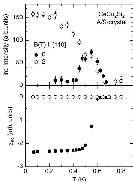
Fig. 3: Temperature dependence of the intensity of a magnetic superstructure peak and the ac susceptibility in an A/S-type  $\text{CeCu}_2\text{Si}_2$  single crystal for  $B = 0$  and 2 T ( $B \parallel [1\bar{1}0]$ ).
